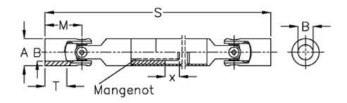
$\begin{array}{lll} A & = 20 \\ B \ H7 & = 12 \\ Longitudinal \ ribs = 6x11x14 \\ M & = 31 \\ MD \ max \ N \ m & = 15 \\ s & = 194 \\ T & = 18 \\ x & = 40 \\ \end{array}$
